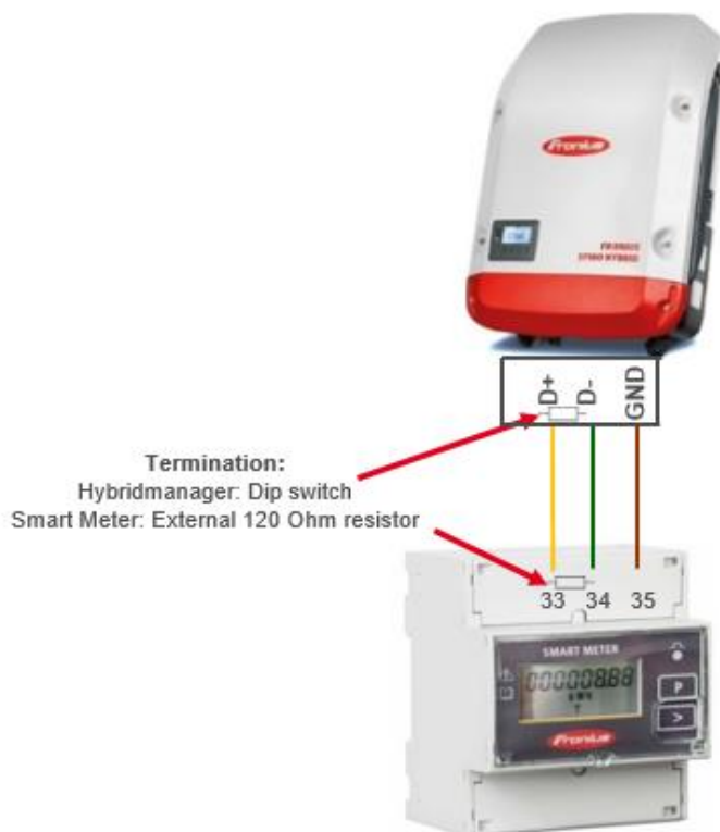
Graphic 4: Modbus connectors and termination
